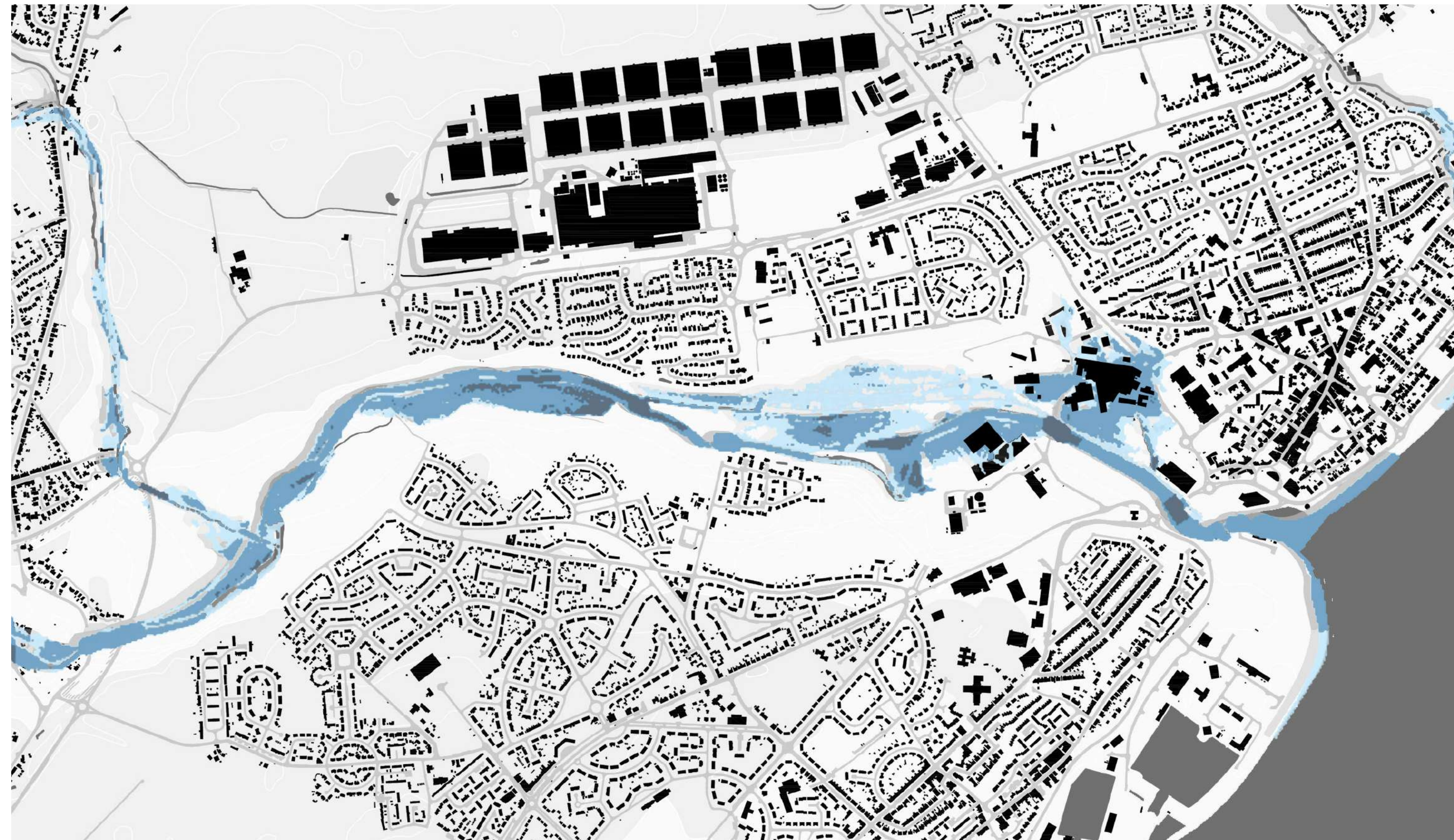
High likelihood depth of fluvial flooding in Connectivity Project area (1:10 - Once in every ten years or 10% chance in any given year)
